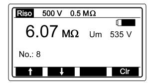
Fig. 103. Example of recalled last stored test result
