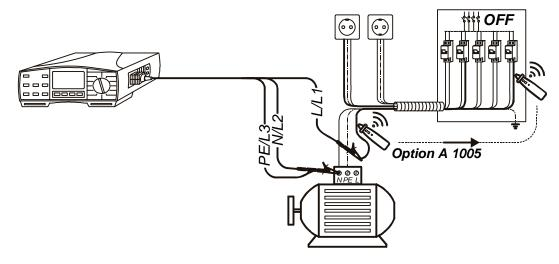
Fig. 86. Connection of Universal Test Cable to a voltage-free conductor
