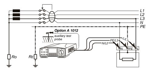
Fig. 42. Connection of Universal Test Cable, measurement with or without auxiliary test probe connected via optional Probe Test Lead (Order No. A 1012)
