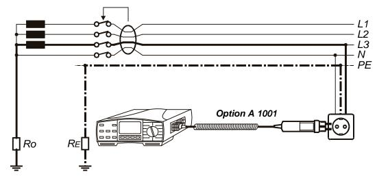
Fig. 59. Connection of optional Plug Commander (Order No. A 1001)
