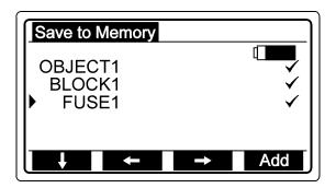
All measurements attached (by means of PC SW only) to the measurement place are already carried out and results stored. Measurer can thus verify any time which measurements have not been done yet and where.
