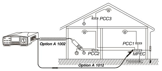
Fig. 16. Connection of optional Tip Commander (Order No. A 1002) and optional Probe Test Lead (Order No. A 1012)
