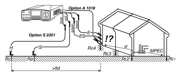
Fig. 29. Connection of optional Earth Test Set – 20 m (Order No. S 2001) and optional Low-range Current Clamp (Order No. A 1018)
