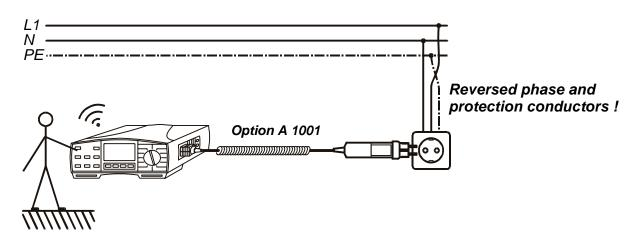
Fig. 38. Connection of optional Plug Commander (Order No A 1001) to mains outlet with reversed L and PE conductors
