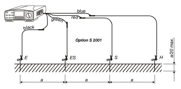
Fig. 36. Connection of optional Earth Test Set – 20 m (Order No. S 2001)
