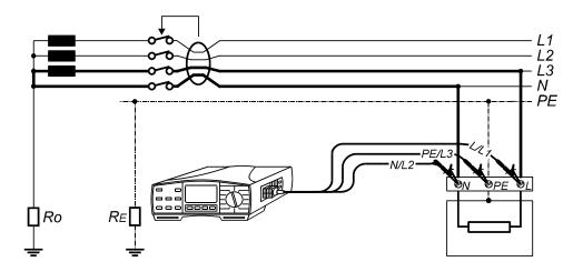
Fig. 70. Connection of Universal Test Cable
