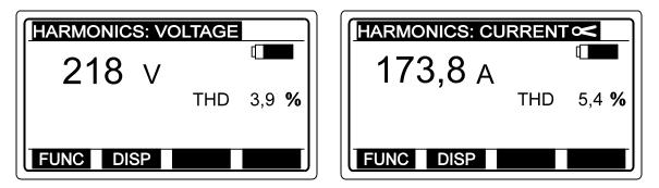
*Fig. 96.* Example of displayed result (THD and effective value of tested Voltage / Current)
