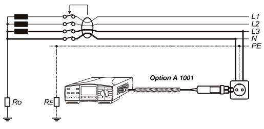
Fig. 65. Connection of optional Plug Commander (Order No. A 1001)
