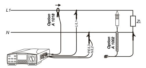
Fig. 90. Connection of optional Low-range Current Clamp (Order No. A 1018) in combination with Universal Test Cable or opt. Tip Commander (Order No. A 1002)
