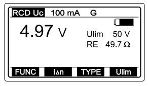
RE (Earth Resistance) is displayed meaning auxiliary test probe has been used. In that case Uc is measured with respect to auxiliary test probe (real ground).
