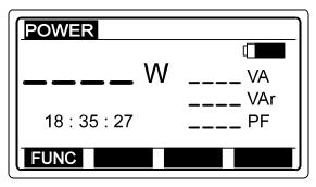
W.....Active power VA .....Apparent power. Var .....Reactive power. PF .....Power Factor.
