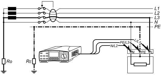
Fig. 60. Connection of Universal Test Cable
