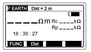
Rc... Resistance of current probe. Rp... Resistance of potential probe.
