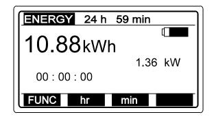
Fig. 93. Example of final energy result
