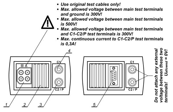
Fig. 2. Connector panel
