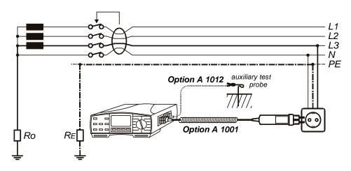
Fig. 41. Connection of optional Plug Commander (Order No. A 1001), measurement with or without auxiliary test probe connected via optional Probe Test Lead (Order No. A 1012)
