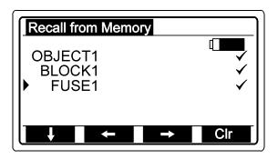
All measurements attached (by means of PC SW only) to the measurement place are already carried out and results stored.
