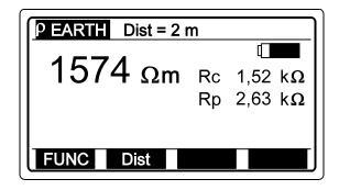
Fig. 37. Example of Earth Resistivity test result
