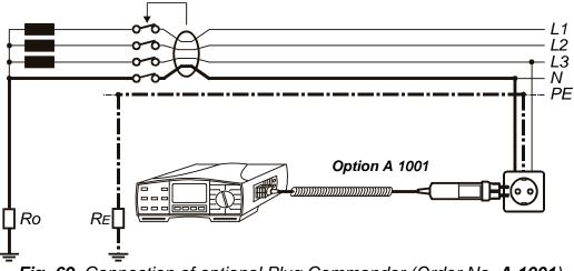
Fig. 69. Connection of optional Plug Commander (Order No. A 1001)
