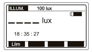
Fig. 81. Illumination measurement initial menu
