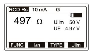
UE is displayed meaning auxiliary test probe has been used. In that case Uc is measured with respect to auxiliary test probe (real ground) and present Rs result is equal to Earth Resistance value.
