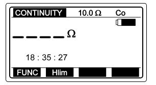
10.0 Ω....Latest set high limit value. Co.....Resistance of test leads has already been compensated in R±200mA function.
