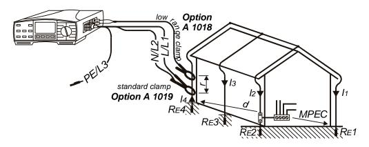
**Fig. 32.** Connection of optional Standard-range Current Clamp (Order No. **A 1019**) using Universal Test Cable and opt. Low-range Current Clamp (Order No. **A 1018**)
