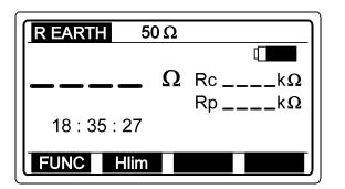
Rc... Resistance of current probe. Rp... Resistance of potential probe.
