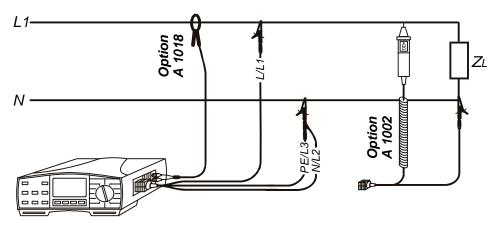
Fig. 95. Connection of optional Low-range Current Clamp (Order No. A 1018) in combination with Universal Test Cable or opt. Tip Commander (Order No. A 1002)
