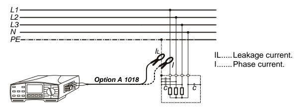
Fig. 76. Connection of optional Low-range Current Clamp (Order No. A 1018)
