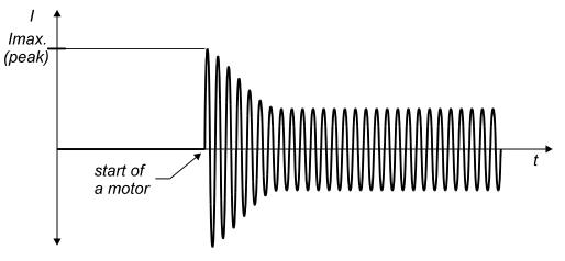
Fig. 78. Motor's start up current
