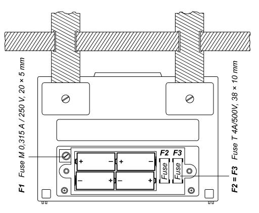
Fig. 104. Correct polarity of inserted batteries
