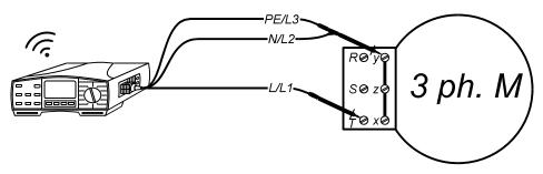
Fig. 20. Connection of Universal Test Cable
