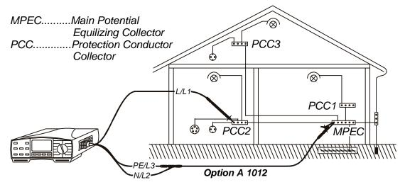
Fig. 15. Connection of Universal Test Cable and optional Probe Test Lead (Order No. A 1012)
