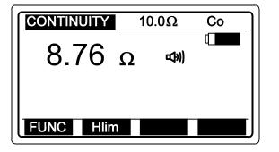
Displayed result is equiped with buzzer sign in case, if it is lower than set high limit value.
