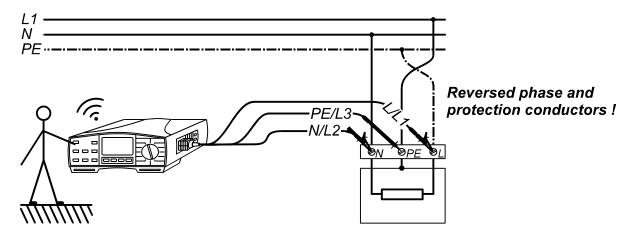
Fig. 39. Connection of Universal Test Cable to load connection terminals with reversed L and PE conductors
