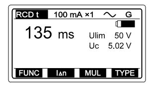
Fig. 48. Example of Trip out time test result
