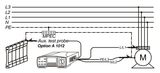
Fig. 62. Connection of Universal Test Cable and auxiliary test probe via optional Probe Test Lead (Order No. A 1012)
