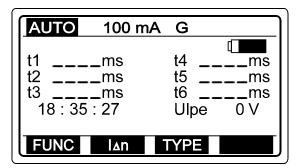
t1 to t6 ... Trip out time of each partial test. Ulpe......Mains voltage between
