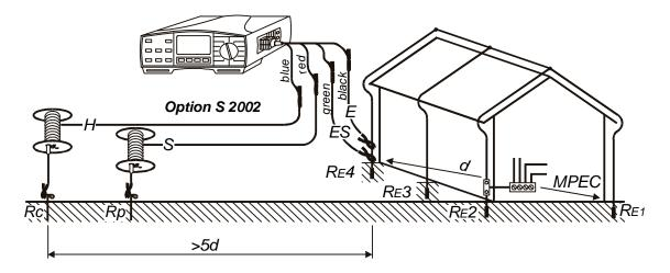
Fig. 26. Connection of optional Earth Test Set – 50 m (Order No. S 2002)
